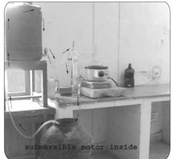
Fig.1 A low cost automated recycling distillation technique Arrows indicate direction of flow of water
